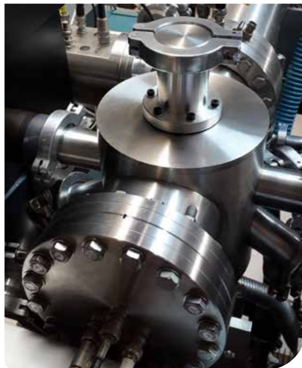
A time-of-flight mass spectrometer is used to measure the masses of the ions that are produced. PHOTO CREDIT: DR CHRISTINE STEENKAMP
