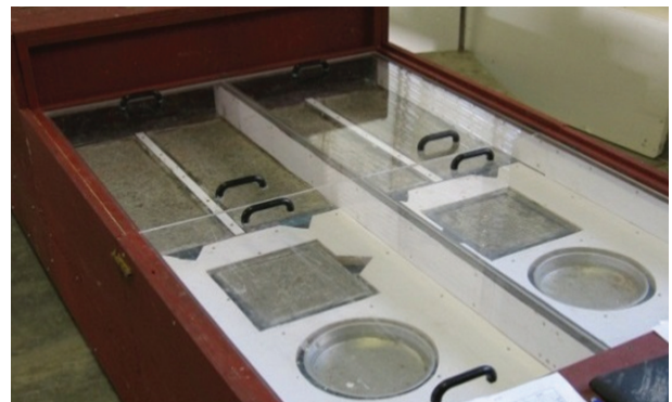
Figure 5. b) the environmental chamber used to quantify the plastic shrinkage cracking.
