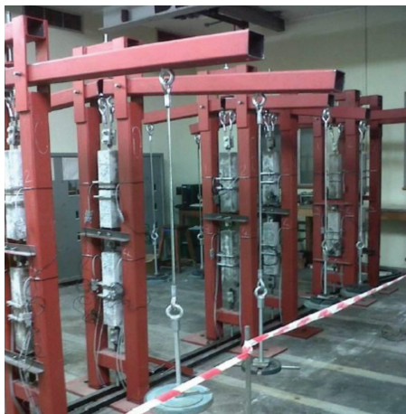
Figure 10. a) The tensile creep test setup.
