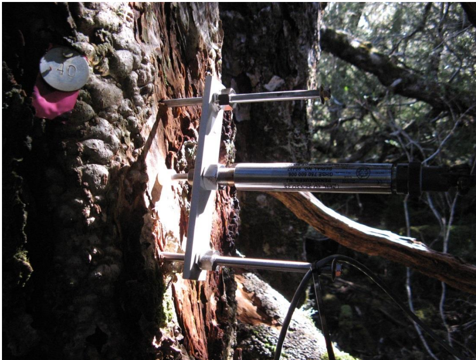
A high resolution electronic point dendrometer measuring stem size variation every 15 minutes on an ancient Huon pine ( Lagarostrobos franklinii ) in western Tasmania, Australia
