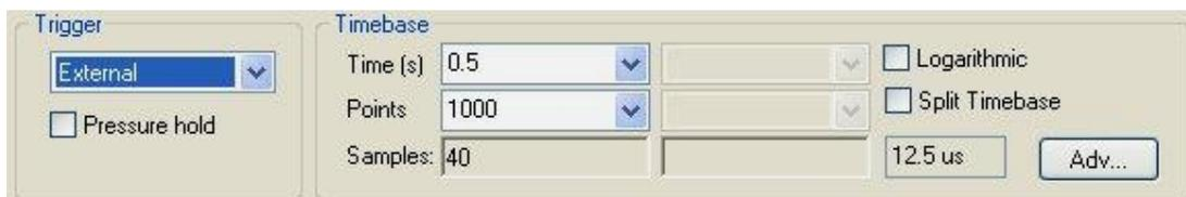
On the **Timebase** panel choose an acquisition time based on the expected timescale of the reaction. **Points** should normally be set to a value between 400 and 1000 data points.
