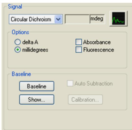
If you wish to record the absorbance simultaneously with the circular dichroism, tick the **Absorbance** box. In this mode the absorbance will not be measured directly, but will be derived from the known change in gain in the Chirascan electronics. The fluorescence can also be recorded by ticking the **Fluorescence** box, but this requires a second (fluorescence) detector.
