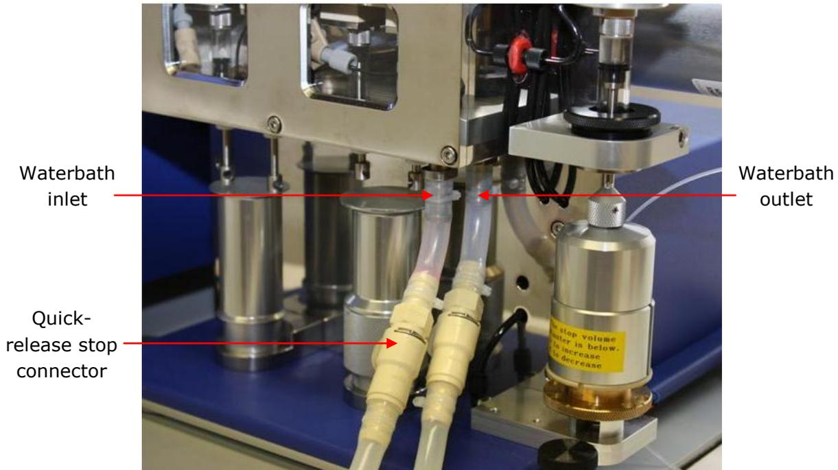
Figure 5.6: waterbath to circulator connections
