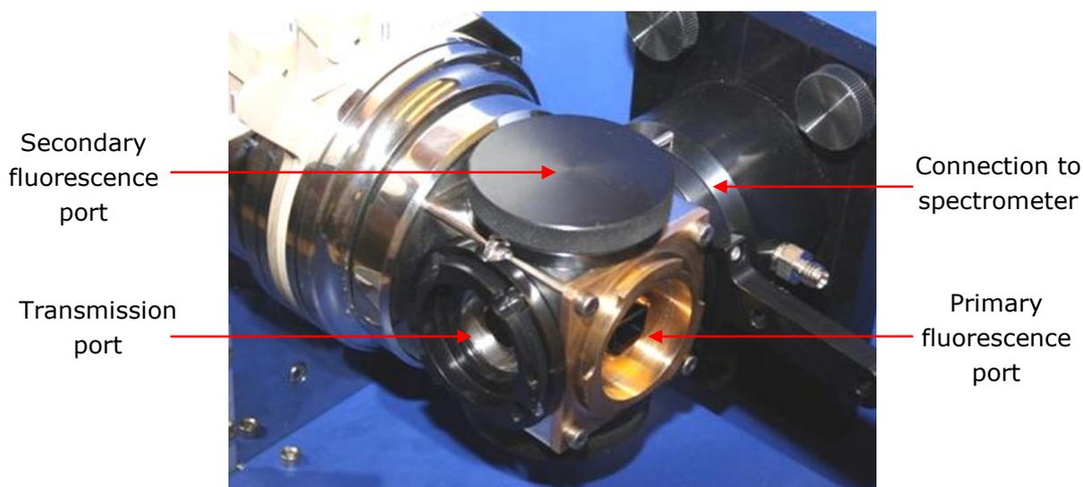
Figure 5.11: detector ports
