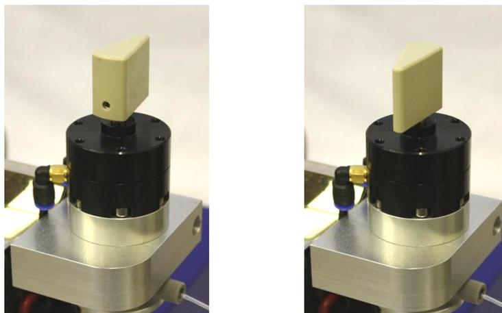
Figure 3.15: the stop valve control knob in the **Drive** position (left) and **Waste** position (right)
