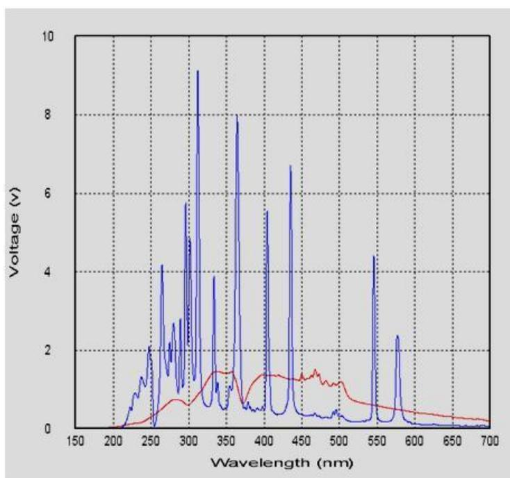
Figure 4.1: comparison of the emission profiles of Hg-Xe (blue) and xenon (red) lamps
