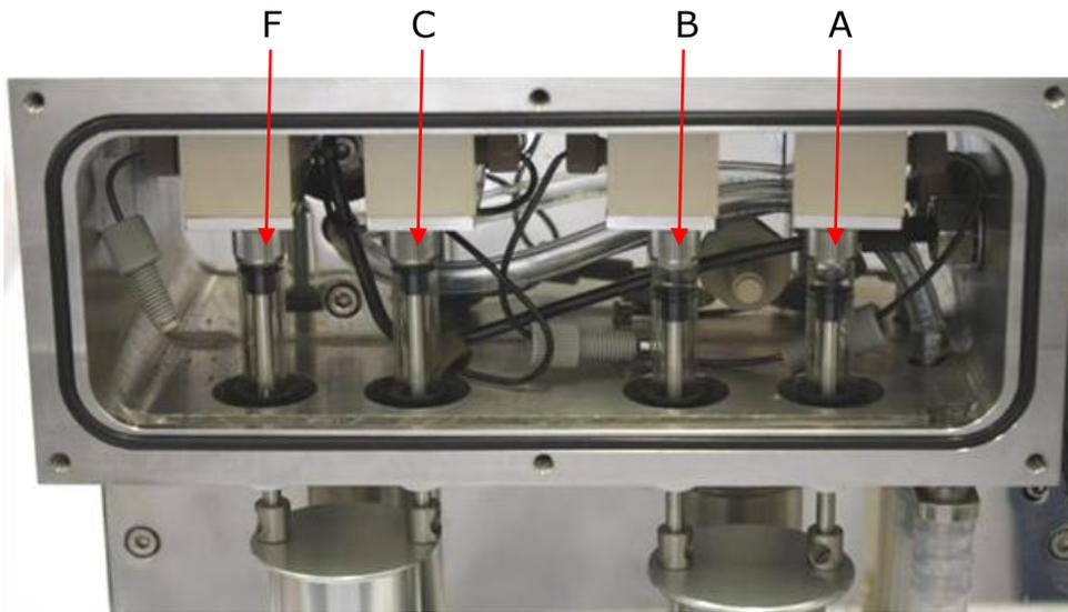
Figure 3.5: the drive syringes in position: for clarity the flow tubing connectors have been removed. Syringes are labelled A, B, C and F (flush) from right to left.
