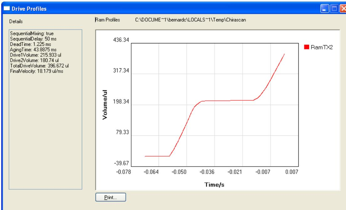
Figure 7.4: sequential-mix drive profile with 50 ms delay time
