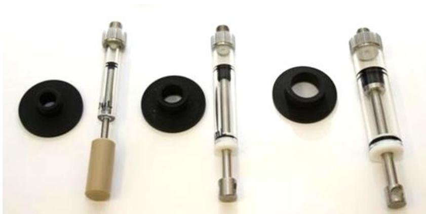
Figure 3.4: 250  $\mu$ L, 1 mL and 2.5 mL drive syringes (left to right), with their respective grommets.
