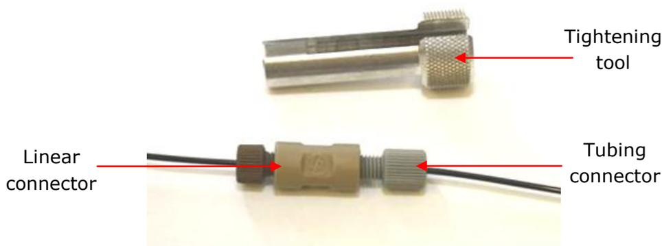
Figure 3.9: tubing connection and tightening tool
