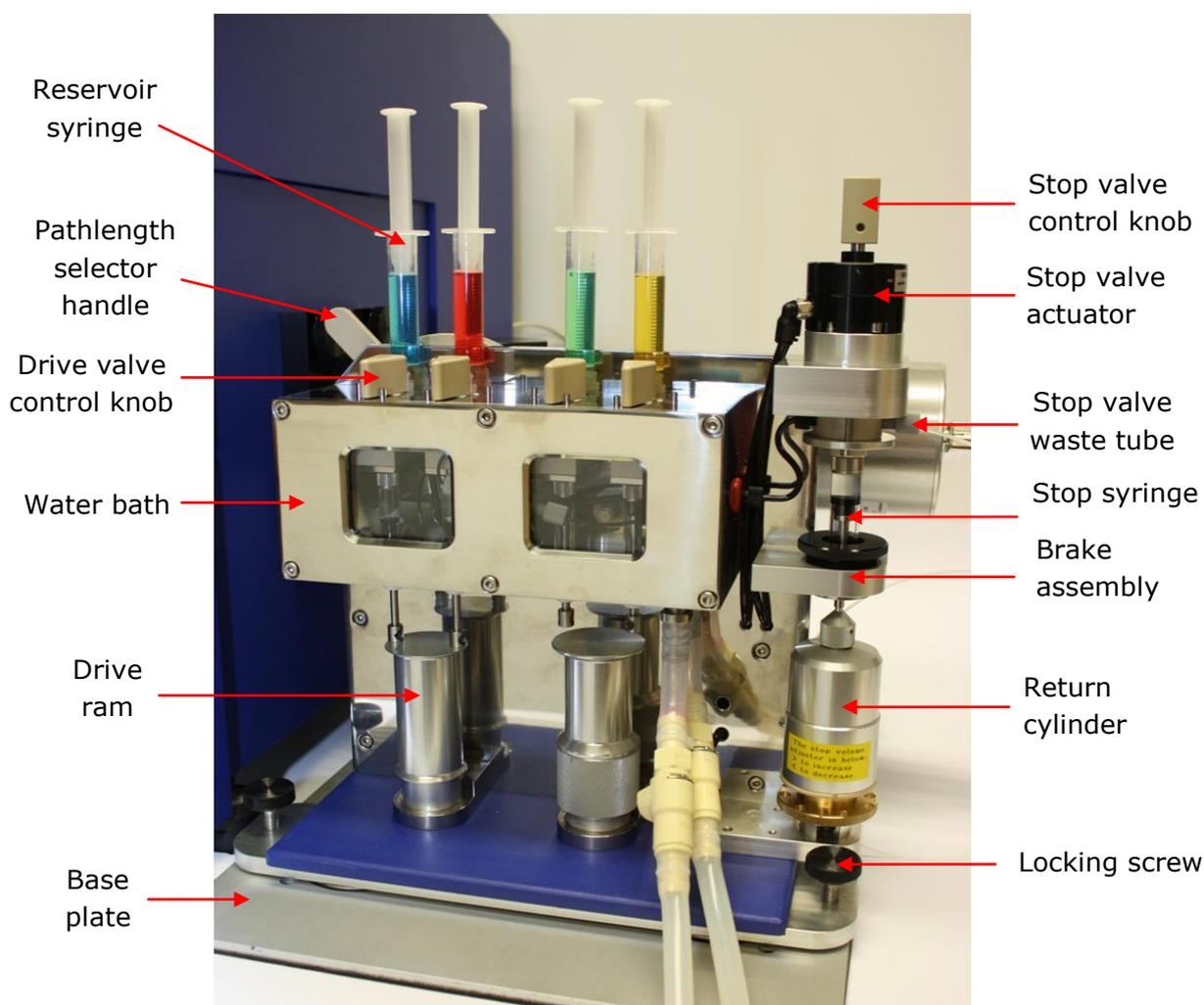
Figure 3.1: the fully assembled SF.3 mounted on the Spectrometer.
