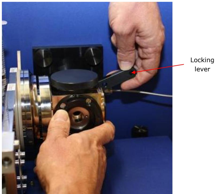
Figure 5.3: the male connector on the SF.3 being eased into the female on the Spectrometer, while the locking lever is held in the Unlock position
