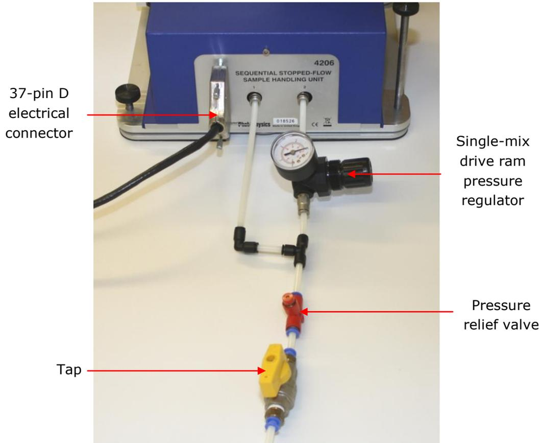
Figure 5.4: electrical and pneumatic connections to the rear of the SF.3 unit
