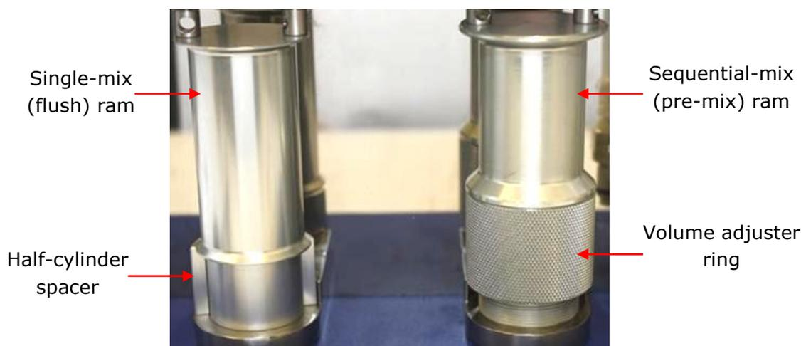
Figure 3.2: single-mix (left) and sequential-mix (right) drive rams. The half-cylinder spacer shown in place on the single-mix ram platform should be removed for single-mixing operation.
