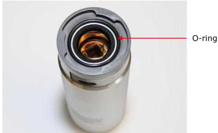
Figure 5.12: PMT detector showing female breech lock connector and O-ring; the O-ring should be removed if an optical filter is fitted.
