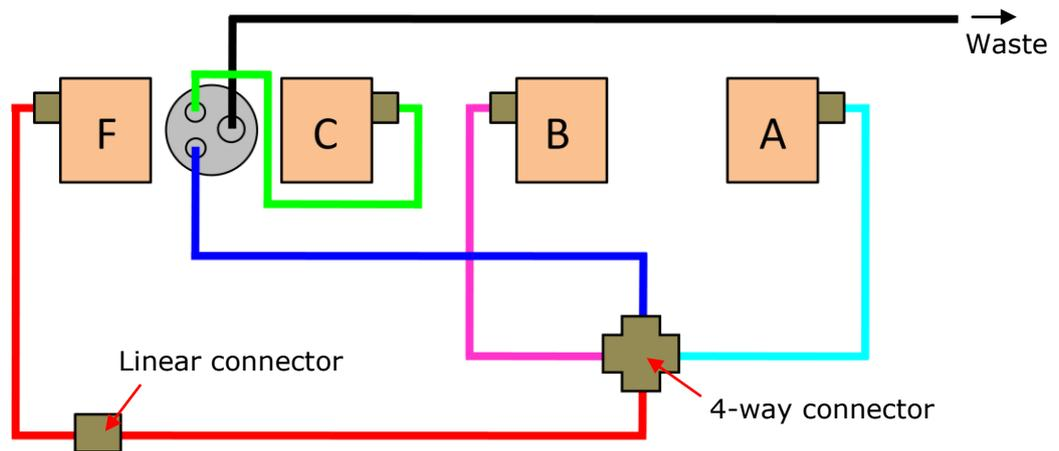
Figure 5.10: schematic of the flow tubing connections for sequential-mix operation; the tubing sections are shown colour coded for clarity
