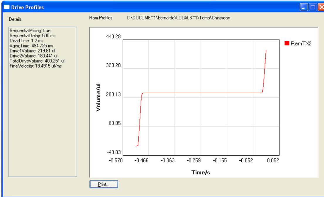
Figure 7.3: sequential-mix drive profile with 500 ms delay time
