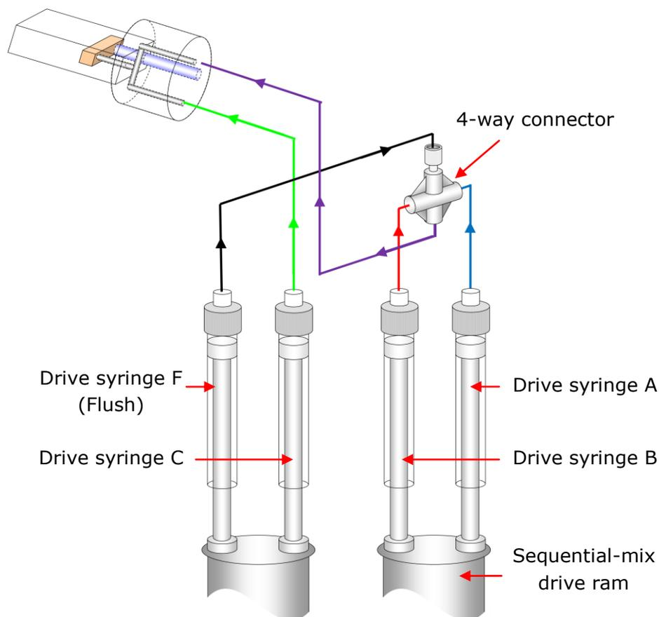
Figure 2.2: schematic of the set-up of the SF.3 for sequential-mixing operation (components of the Auto-Stop assembly are omitted for clarity)
