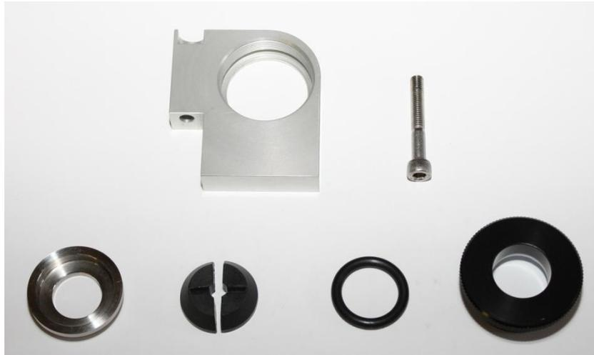
Figure 3.16: components of the brake assembly: left to right, top: mounting plate and screw; bottom: seating ring, brake shoes, O- ring, knurled retaining ring.
