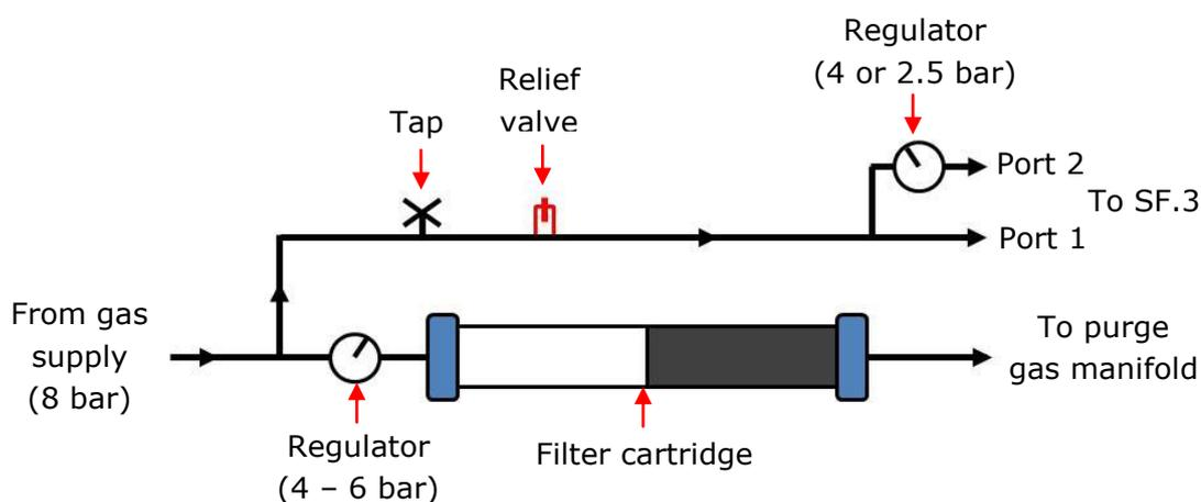
Figure 5.6: schematic of the pneumatic and filter connections
