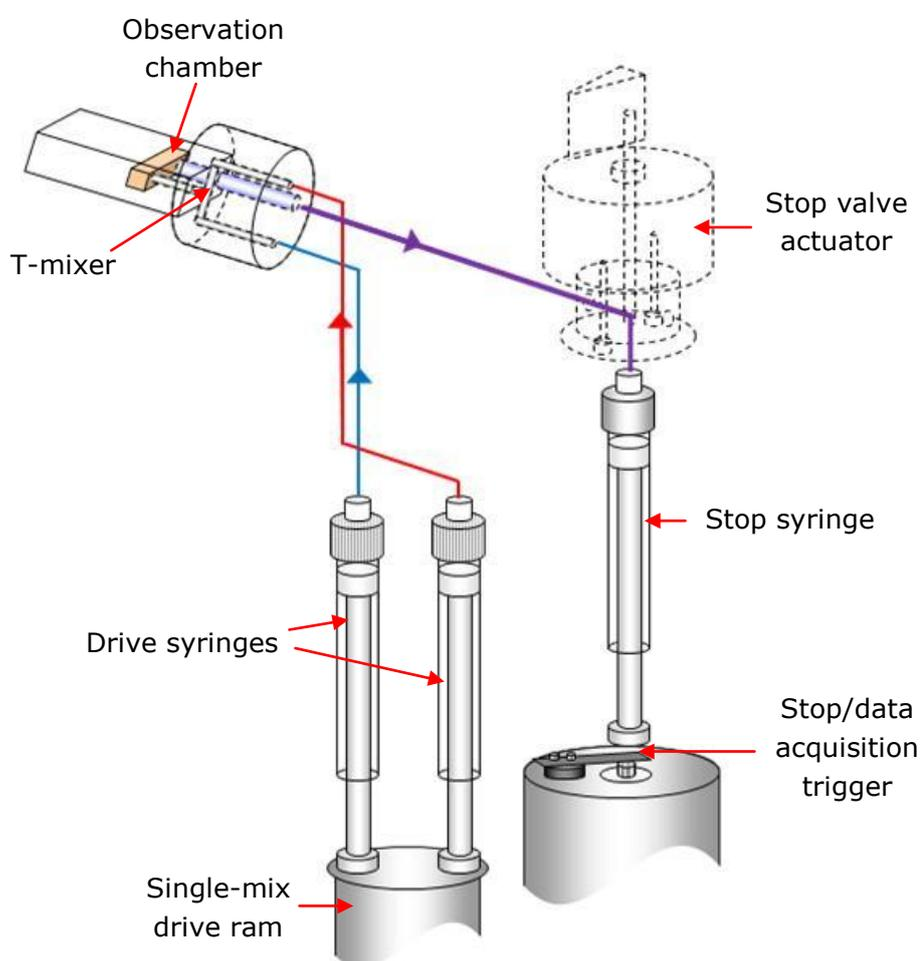
Figure 2.1: schematic of the set-up of the SF.3 for single-mixing operation
