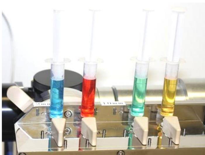
Figure 3.6: reservoir syringes mounted on the SF.3. All four syringes are used for sequential-mixing; only syringes C and F are used for single-mixing
