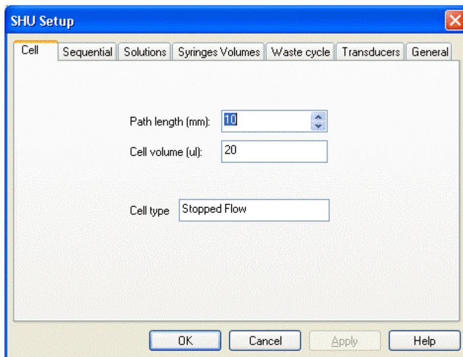
Figure 6.4: the Cell tab
