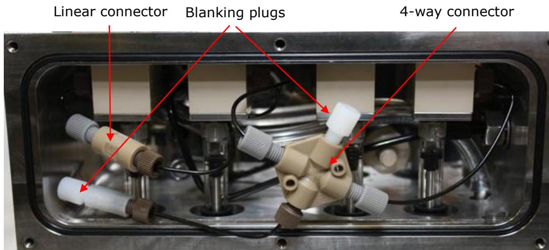
Figure 5.7: flow tubing connections for single-mix operation
