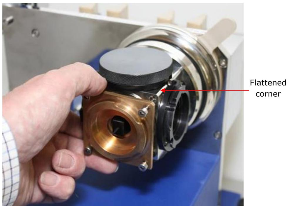
Figure 3.13: removal of the cell cartridge by withdrawal from the rear of the SF.3 unit
