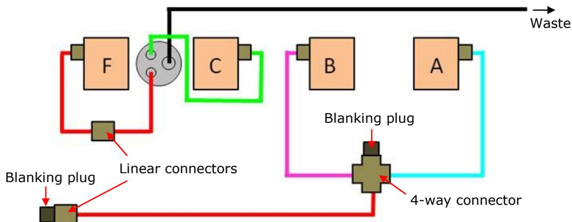
Figure 5.8: schematic of the flow tubing connections for single-mix operation; the tubing sections are colour coded for clarity
