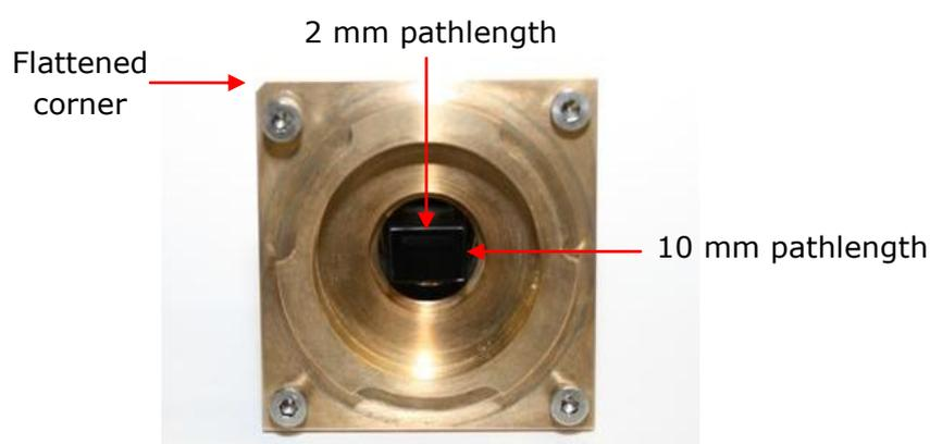
Figure 3.12: detail of the cartridge fluorescence port
