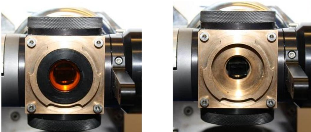
Figure 5.15: primary fluorescence port with the optical filter in place (left) and removed (right).
