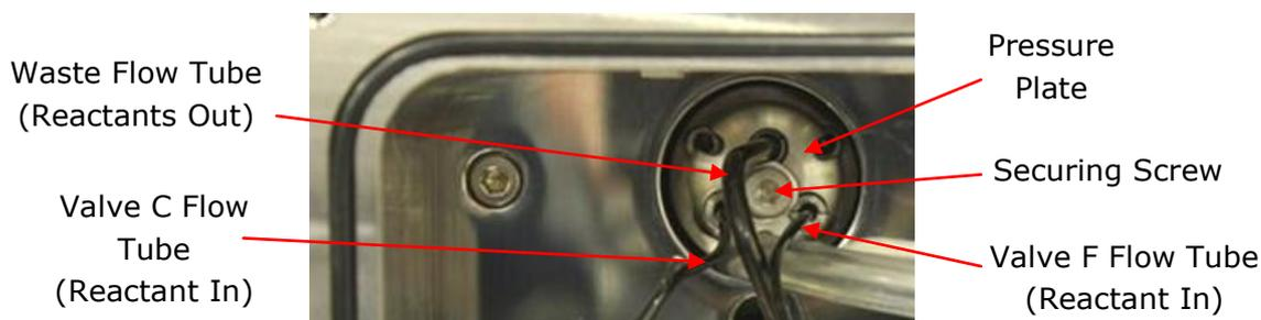
Figure 3.8: the arrangement of the pressure plate and flow lines when the pathlength is set to 2 mm. For clarity the drive valves and syringes have been removed.
