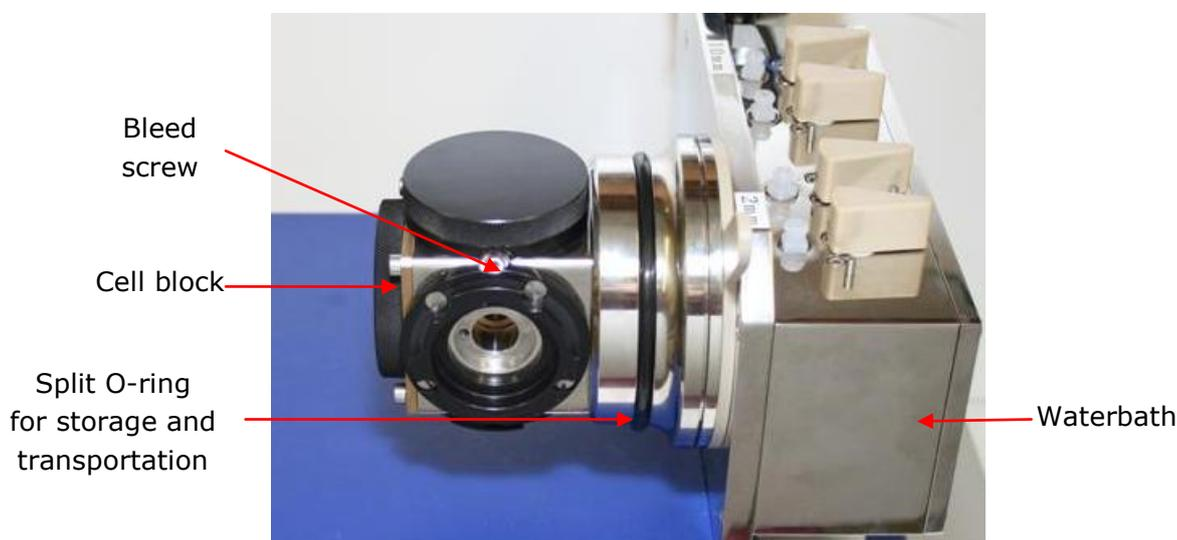
Figure 3.3: the SF.3 waterbath and cell block. The split O-ring should be removed before the SF.3 is installed on the spectrometer
