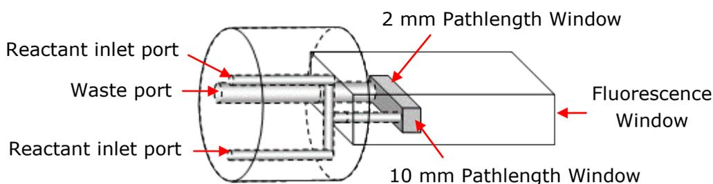
Figure 3.10: schematic of the internal design of the 20  $\mu\text{l}$  optical cell.
