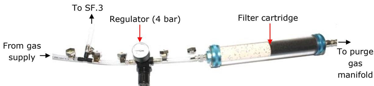
Figure 5.5: pneumatic and filter connections for a single gas source
