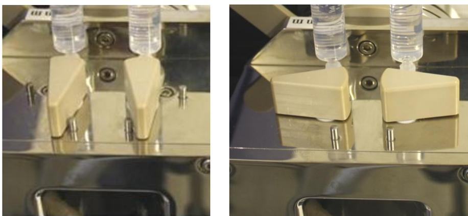
Figure 3.7: drive valves set to the Drive position (left) and Load position (right)
