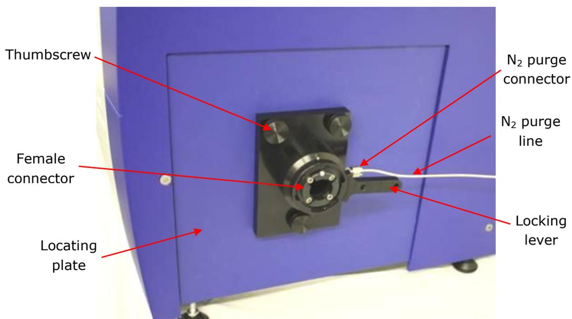
Figure 5.1: the SF.3 locating plate mounted on the Chirscan
