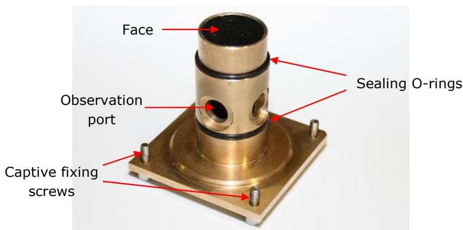
Figure 3.11: the cell cartridge
