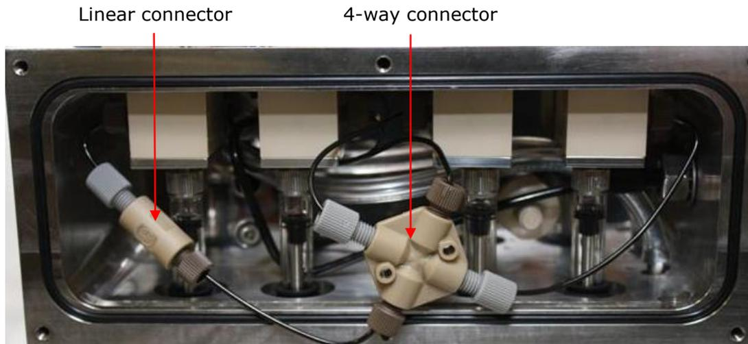
Figure 5.9: flow tubing connections for sequential-mix operation
