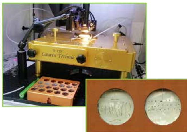
**Figure. 13:** Resin-mounted gold shavings and grains placed in the laser ablation sample cell.
