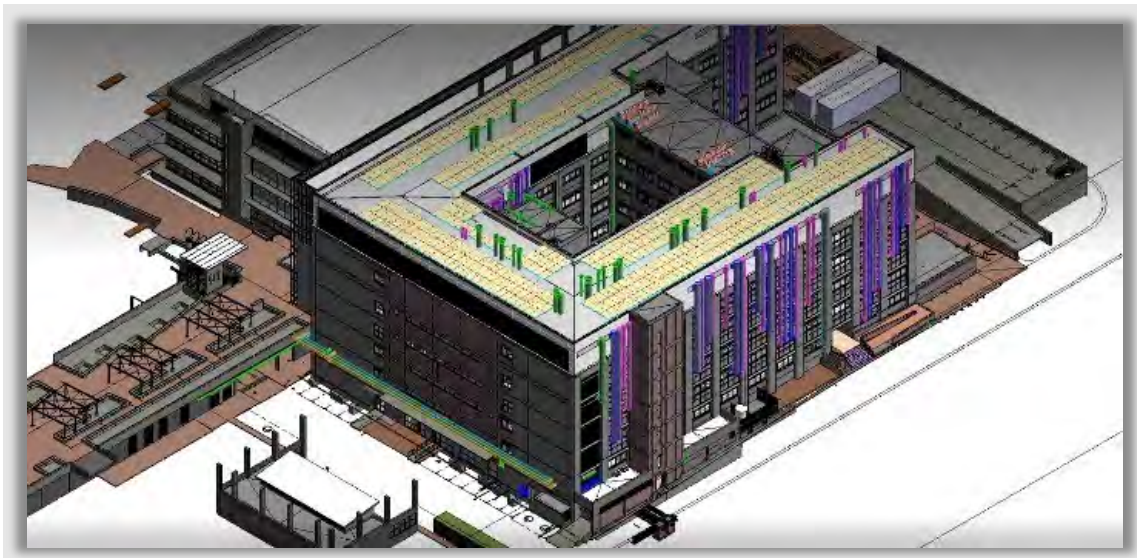
Figure 24: This image of the Natural Science is a Scan to BIM of an Existing Building.
