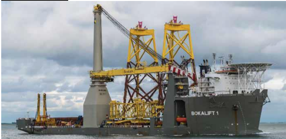
The Bokalift 1 outbound from Vlissingen loaded with 2 jackets for installation Photo : Henk Nagelhout ©
