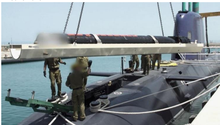
A still from a video released by the IDF shows a Kaved torpedo being loaded into a submarine at the Haifa naval base. Source: Israel Defense Forces
