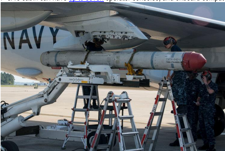
Crew members load an AGM-84K SLAM-ER missile on a P-8A Poseidon, April 4, 2014. US Navy photo by Mass Communication Specialist 3rd Class Jason Kofonow
