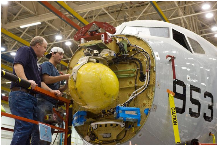
Boeing and Raytheon employees complete installation of an APY-10 radar antenna on P-8A Poseidon test aircraft T2, November 2009. Boeing
