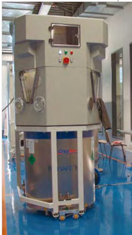
The cryostorage tank is equipped with a special access tower (above) with computer control for the deposit and retrieval of the HI virus samples.
