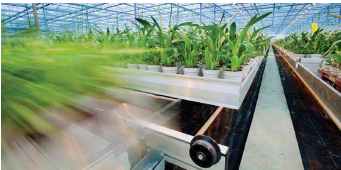
Top: Mechanical harvesting of cherries; experimental unit in Michigan, USA. Above: Automated tray transfer in greenhouses. PHOTO: WAGENINGEN UR GREENHOUSE HORTICULTURE, THE NETHERLANDS
