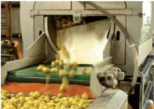
Washed and 'polished' potatoes exit this machine at the rate of 15 tonnes per hour. PHOTO: WWW.WYMASOLUTIONS.COM
