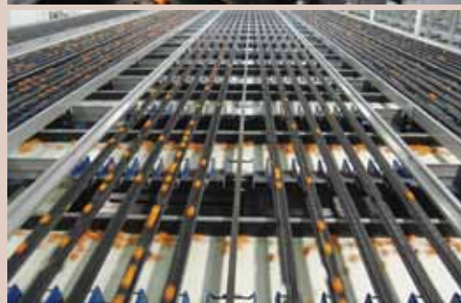
(Upper photo) In California a bank of high speed grading machines micro weigh and photo stitch analyse mandarins for blemishes across 40 lanes at 10 fruit per second per lane, and (lower photo) travel at high speed to assigned packing stations. PHOTO: WWW.COMPACSORT.COM
