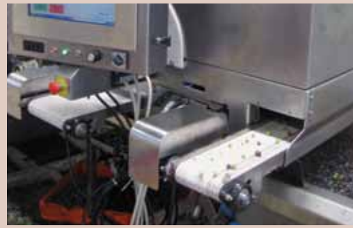
High speed berryfruit grader uses colour sensing technology to identify and air jets to remove non-conforming berries. PHOTO: WWW.BBCTECHNOLOGIES.COM
