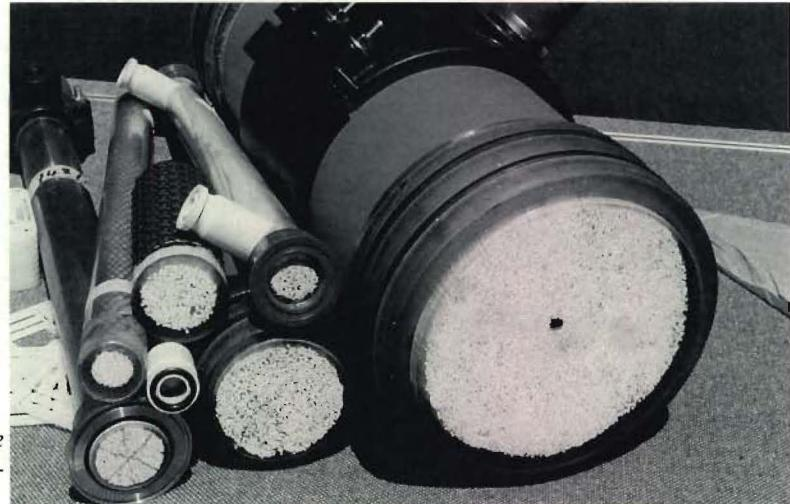
*There is an ever increasing sophistication in the size and design of membrane modules for water sterilization.*
