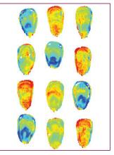
Conventional near infrared (NIR) spectroscopy and NIR hyperspectral imaging are used, in conjunction with chemometrics, for quantitative, qualitative and authentication studies. Advanced image analyses are applied to study spatially resolved hyperspectral images (chemical maps) of food and agricultural products. The newly established Vibrational Spectroscopy Unit of the Central Analytical Facility of SU is housed in the Department.
