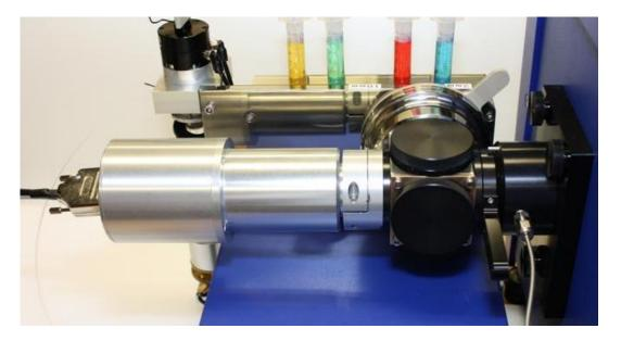
Figure 5.13: a detector installed in the transmission port
