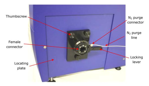
Figure 5.1: the SF.3 locating plate mounted on the Chirascan
