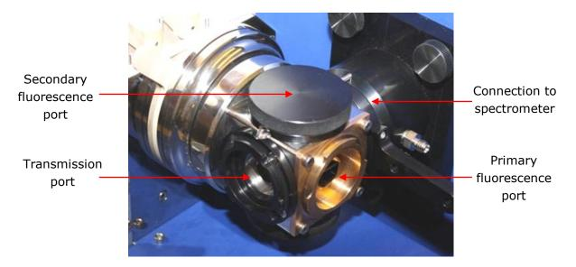
Figure 5.11: detector ports
