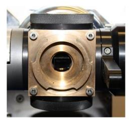
Figure 5.15: primary fluorescence port with the optical filter in place (left) and removed (right).
