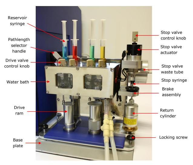
Figure 3.1: the fully assembled SF.3 mounted on the Spectrometer.
