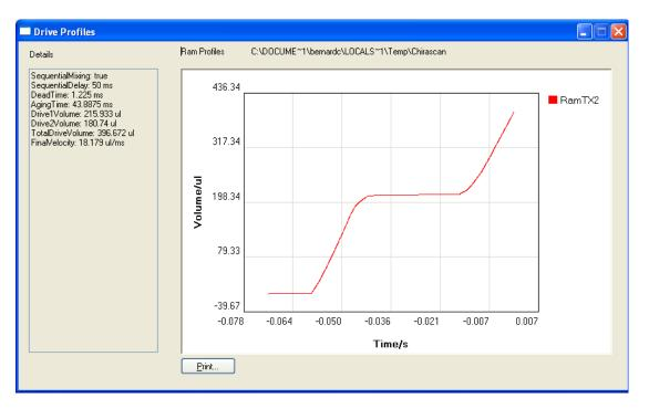
Figure 7.4: sequential-mix drive profile with 50 ms delay time
