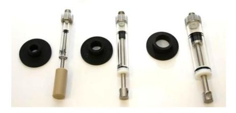
Figure 3.4: 250  $\mu\text{L},$  1 mL and 2.5 mL drive syringes (left to right), with their respective grommets.
