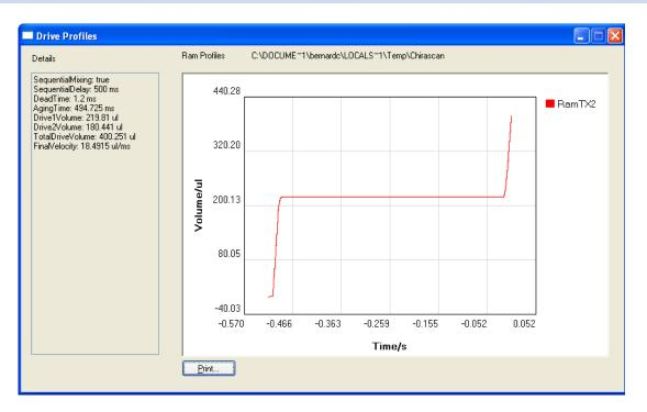
Figure 7.3: sequential-mix drive profile with 500 ms delay time
