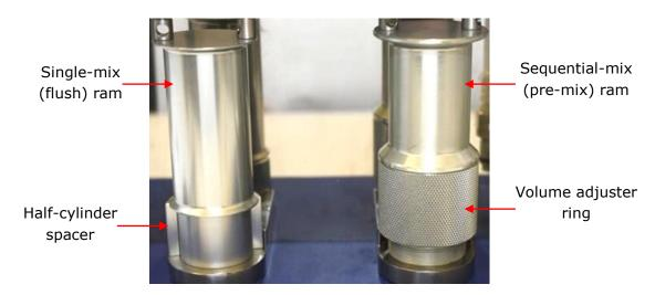
Figure 3.2: single-mix (left) and sequential-mix (right) drive rams. The half-cylinder spacer shown in place on the single-mix ram platform should be removed for single-mixing operation.
