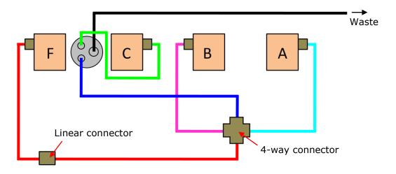
Figure 5.10: schematic of the flow tubing connections for sequential-mix operation; the tubing sections are shown colour coded for clarity
