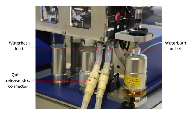
Figure 5.6: waterbath to circulator connections
