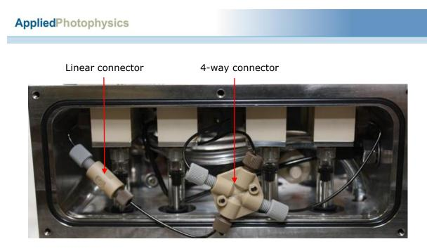
Figure 5.9: flow tubing connections for sequential-mix operation
