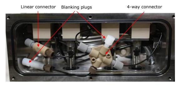
Figure 5.7: flow tubing connections for single-mix operation
