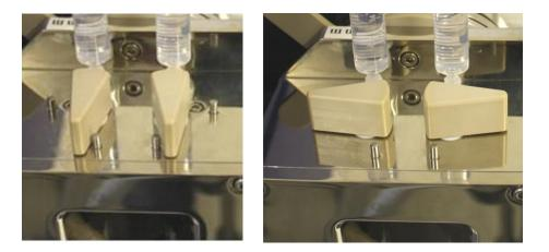
Figure 3.7: drive valves set to the Drive position (left) and Load position (right)
