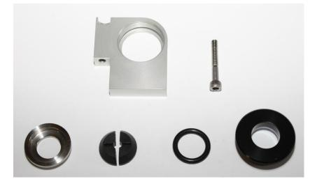
Figure 3.16: components of the brake assembly: left to right, top: mounting plate and screw; bottom: seating ring, brake shoes, O- ring, knurled retaining ring.
