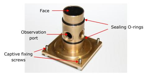
Figure 3.11: the cell cartridge
