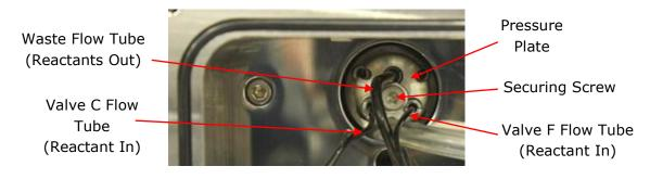
Figure 3.8: the arrangement of the pressure plate and flow lines when the pathlength is set to 2 mm. For clarity the drive valves and syringes have been removed.
