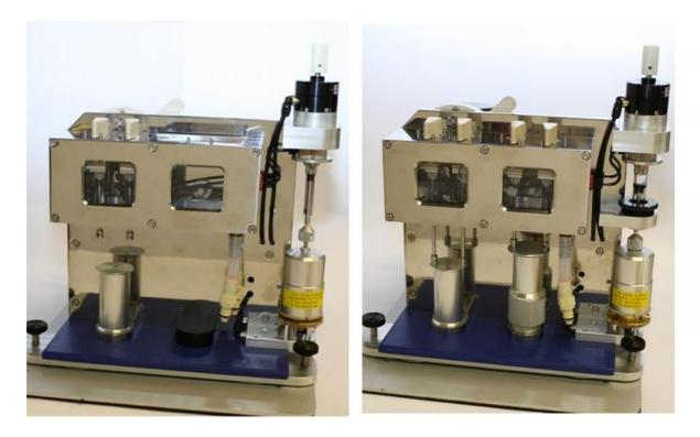
Figure 1.1: The single mixing (left) and sequential mixing (right) versions of the SF.3
