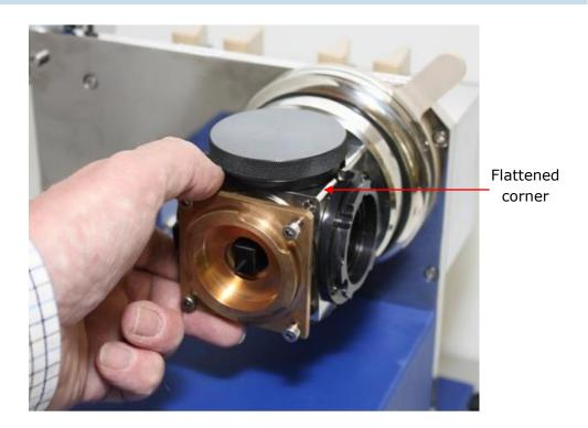
Figure 3.13: removal of the cell cartridge by withdrawal from the rear of the SF.3 unit
