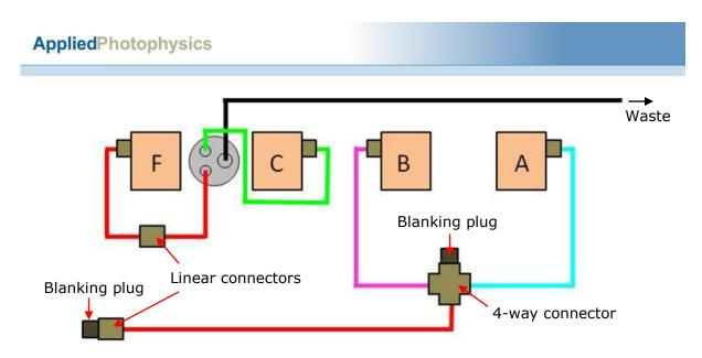
Figure 5.8: schematic of the flow tubing connections for single-mix operation; the tubing sections are colour coded for clarity
