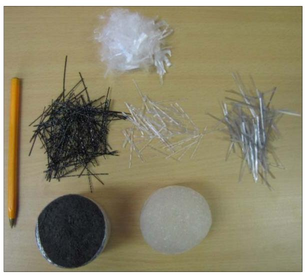
Figure 2. 2: Examples of polypropylene micro- and macro fibres.
