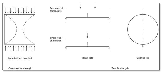
Figure 2.3: Tests to measure the strength of concrete (Fultons 9<sup>th</sup> edition, 2009).
