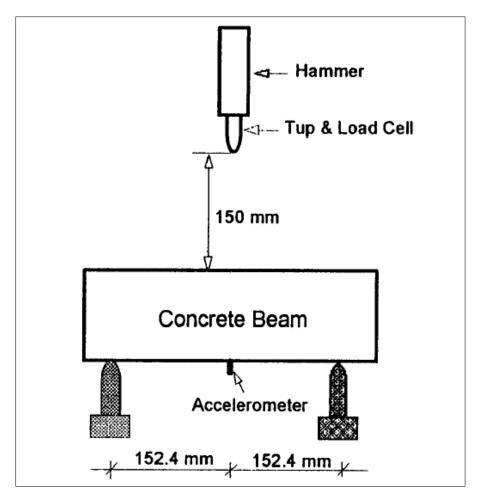
Figure 2.10: Impact load test setup (Wang & Mindess & Ko, 1996).
