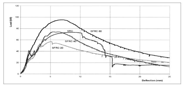
Figure 2.6 Comparison of SRC to SFRC for different fibre dosages at an age of 48h (Ding & Kurnele, 1999).
