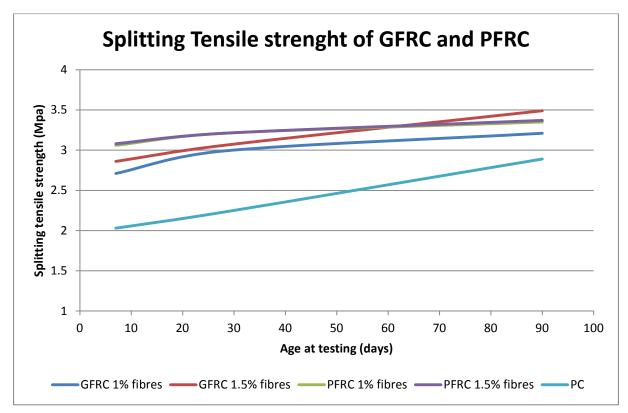
Figure 2.8: Comparison of splitting tensile strength of GFRC and PFRC with unreinforced concrete after Choi & Yuan (2004).
