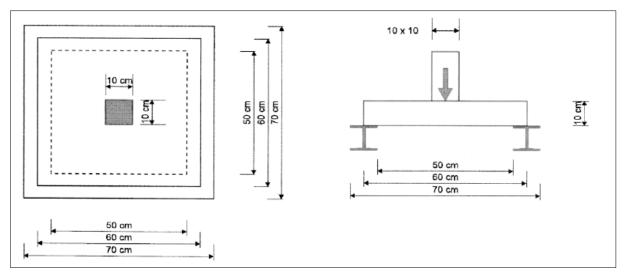
Figure 2.4 Test set setup for panel tests according to EFNARC (Ding & Kurnele, 1999).
