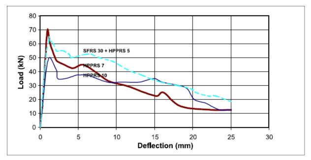
Figure 2.7: Comparison of hybrid fibre reinforcement to HPPFR (Cengiz & Turanli, 2004).
