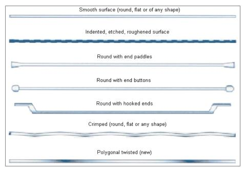
Figure 2.1: Steel fibre geometries (Concrete Society UK TR 63, 2007).
