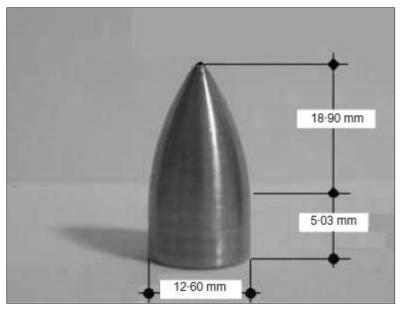
Figure 2.11: Projectile for impact testing (Zhang & Sharif & Lu, 2007).
