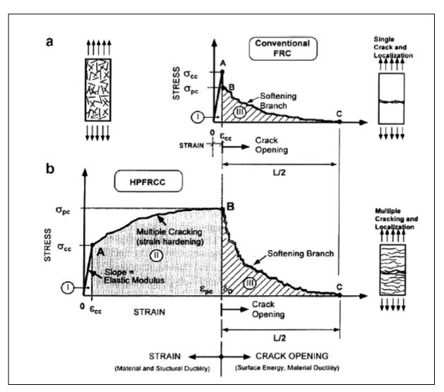
Figure 2 5: Strain hardening and strain softening behaviour of different FRC's (Brandt, 2008).
