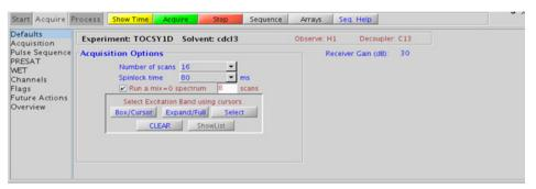
• The zTOCSY1D experiment contains a zero-quantum filter to suppress artifacts and often gives better results than the TOCSY1D.
