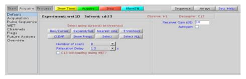
If a PROTON spectrum has not been previously acquired but the "Select Later" and "Do Scout" options were checked on the "Default" panel shown in the "Key parameters" sections, the scout scan is acquired and the data displayed, now with the "Default" panel shown above to facilitate the interactive peak selection.
