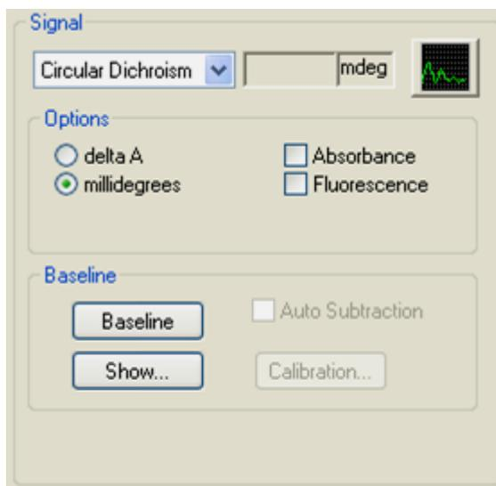
If you wish to record the absorbance spectrum simultaneously with the circular dichroism spectrum, tick the **Absorbance** box. In this mode the absorbance will not be measured directly, but will be derived from the known change in gain in the Chirascan electronics. The fluorescence spectrum can also be recorded by ticking the **Fluorescence** box, but this requires a second (fluorescence) detector.
