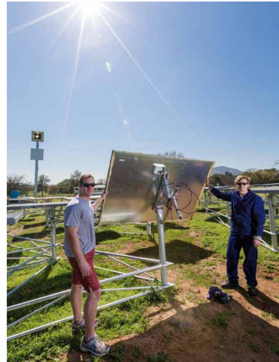
Liam May (coordination assistant) and Willem Landman (design engineer) from the Helio100 team holding a heliostat reflecting sunlight onto the receiver tower.
