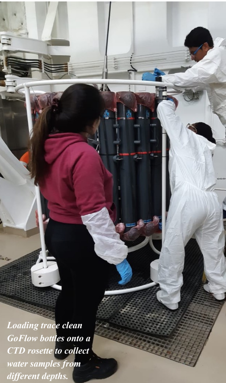
GoFlow bottles brought from clean lab in plastic bags to be loaded onto rosette.
