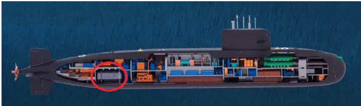
An image released during IDEX 2017 clearly shows an oxygen tank (circled in red) for the Stirling cycle AIP system. (CSOC)
