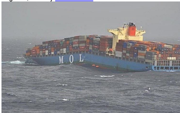
MOL Comfort showing signs of extreme hogging before breaking up in the Indian Ocean in June 2013.
