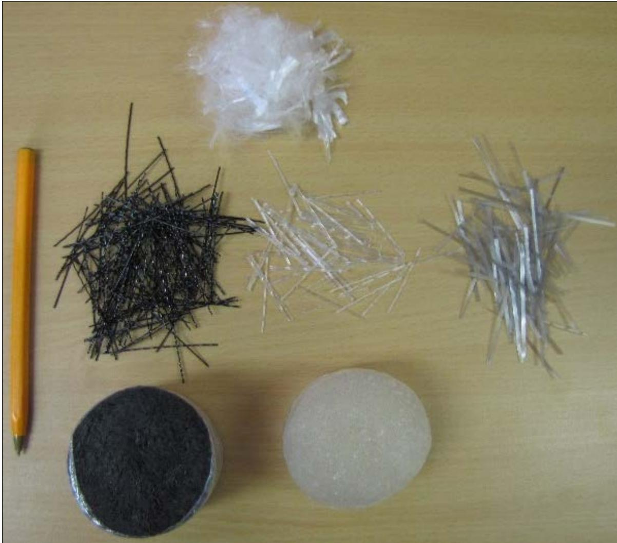
Figure 2. 2: Examples of polypropylene micro- and macro fibres.
