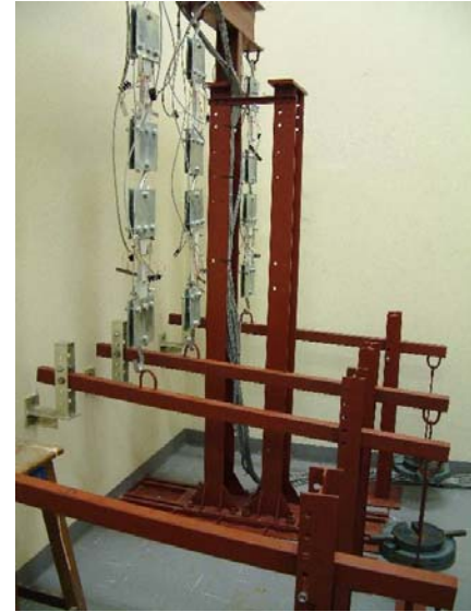
Figure 8: Force controlled uni-axial tensile test setup
