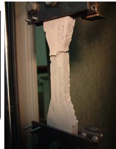
Figure 13: Summary of ultimate resistances of the tensile tests (left) and a typical failure of a ECC specimen.
