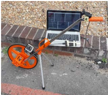
Figure: Experiment hardware setup. 1) USB webcam (Logitech c170 with 640x480 resolution) 2) Measurement wheel 3) GoPro Hero 3 (used for distance scaling) 4) Tape 5) Laptop running LSD-SLAM
