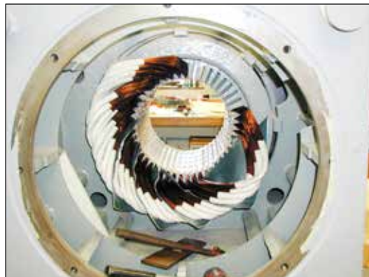
Pietro Petzer's most challenging task: The re-winding of this 300 kW induction machine.
