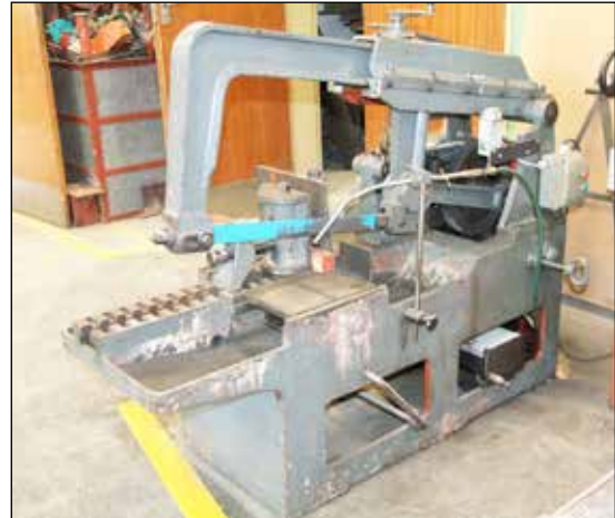
Repairing old equipment means saving money. Here is the heavy duty hacksaw machine of 950 kg manufactured in Italy and purchased by Civil Engineering in 1979 - restored by Dion Viljoen.
