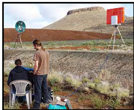
Calibration testing of the IRA using a packaged PCB LPDA and the real time analyser RTA3.
