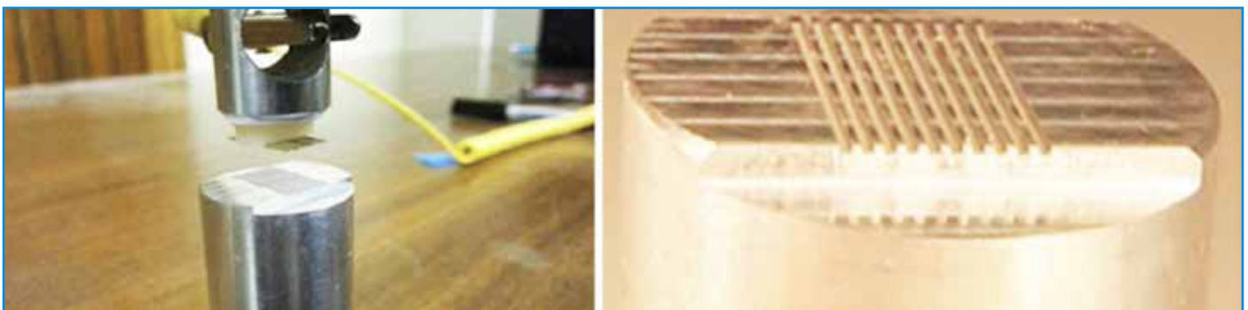
Figure V: Picking and placing of 200 µm bars in a pre-grooved assembly utilising Van der Waals forces.
