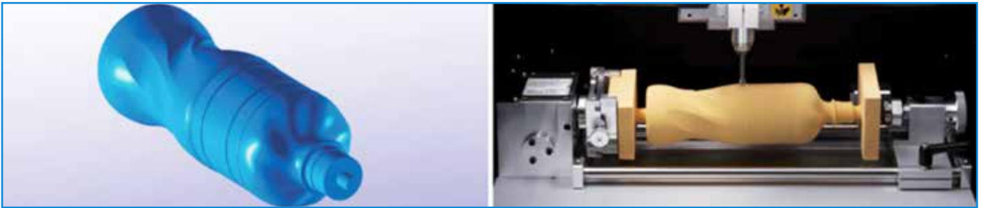
Figure I: Bottle design in CAD shown on the left and the Roland micro-milling manufacturing process on the right.
