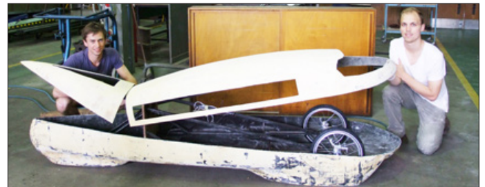
Progress so far: Tian van Tonder and Felix Cranz with the tear-drop-shaped, lightweight, high-strength, carbon fibre hull.
