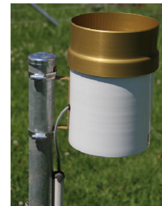
self-emptying tipping bucket rain gauge
